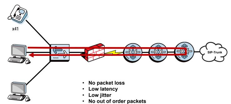
Test round-trip to each segment along the way to isolate
